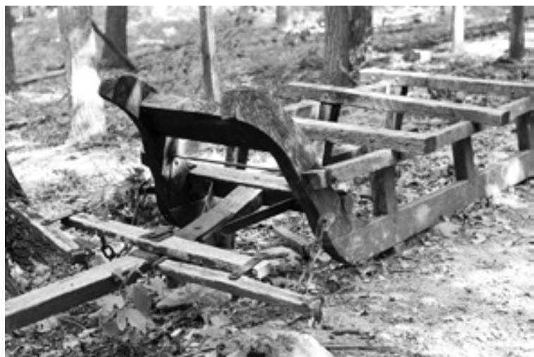
This type of sled was used by timber cutters to haul logs that were made into charcoal to fuel the Catoctin Iron Furnace.
